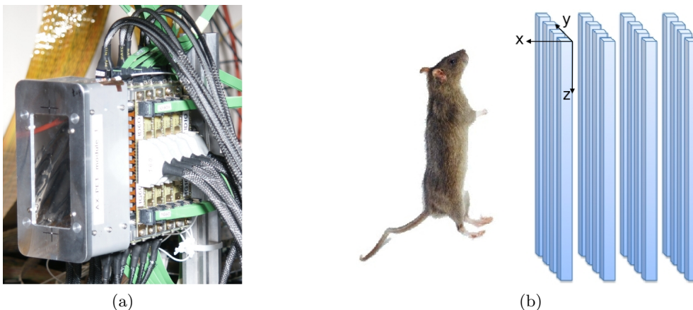
FIG. 15: (a) Photograph of one module of AX-PET demonstrator. (b) Sketch of phantom position with respect to the module.
